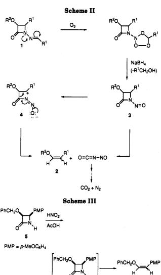
ozonolysis of compounds 1, the results can support N-nitroso- $\beta$ -lactams 3 as probable intermediates in the formation of vinyl ethers 2.
